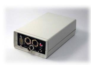
Compact PDA-based I<sup>2</sup>C BUS monitor. Four AA batteries for 8 hours or more. Graphical user interface. Data analysis functionalities. 50708090A0B0C0D0..
